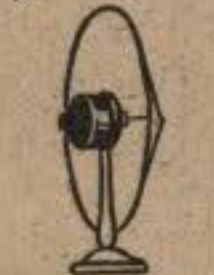
A cone diaphragm loud speaker can easily be constructed. The illustration shows one method of mounting.
